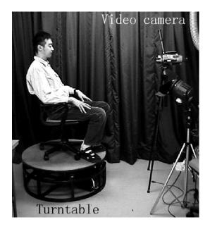
Figure 7. A turntable type image-capturing camera
